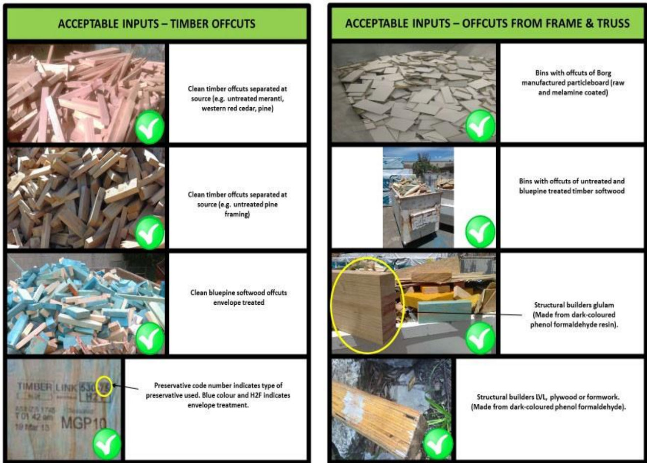
Figure 3.1. Acceptable waste streams for facility – timber offcuts and plasterboard.
